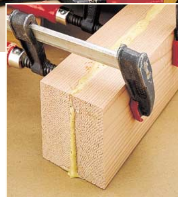
▲ One unique characteristic of polyurethane glue is that it foams as it reacts with the moisture in the wood.
