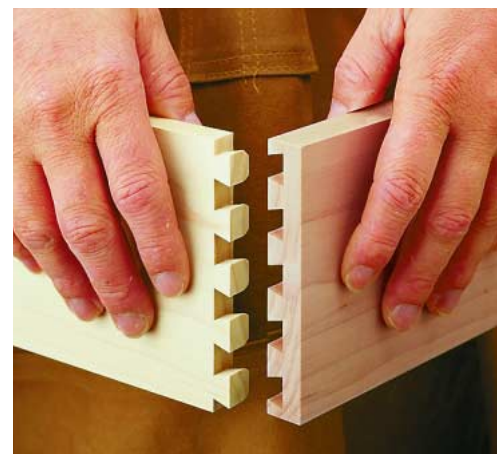
▲ Test fit. With the pieces removed from the jig, test the fit of the joint. The tails should slide halfway into the sockets. A soft mallet can then be used to drive the joint home.
