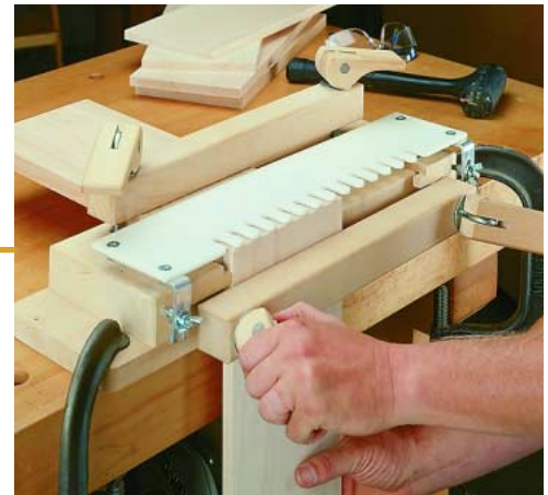
▲ Clamp pieces in jig. After positioning both workpieces underneath the jig template, tighten down the cams on the clamping bars to hold the workpieces securely in place.
