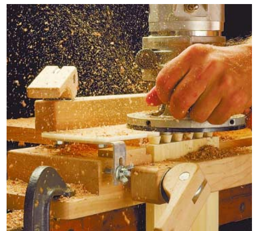
▲ Rout dovetails. The template guides the router in and out as the dovetails and pins are routed simultaneously. This ensures a perfectly-aligned joint every time.
