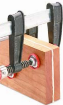
▲ Bracket feet look like they were cut from thick blocks of wood, but these blanks were made with two pieces of ¾"-thick stock.
