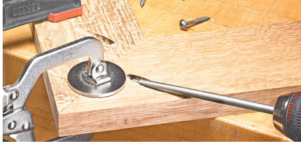
▲ Two pocket holes square to the miter joint and opposite one another allows pocket hole screws to secure the joint. A face frame clamp makes it easy to hold the joint in position while the screws are inserted.
