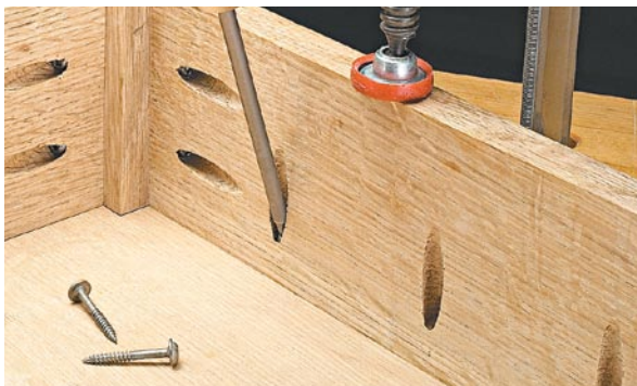
▲ Attach a table top by drilling pocket holes and driving screws. Drilling the pilot hole a bit larger and backing the screw out slightly, allows for wood movement.
