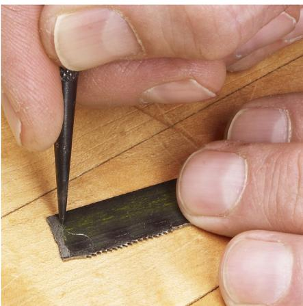
▲ Using a scratch awl, scribe the profile onto a piece of tool steel. Here, I'm using an old hacksaw blade.
