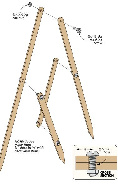
As I discussed in the article on page 48 of *Woodsmith* No. 201, the golden ratio (1.618) can be a very helpful design tool. It gives you a reliable starting point when hashing out the overall proportions of a project and its individual components.
