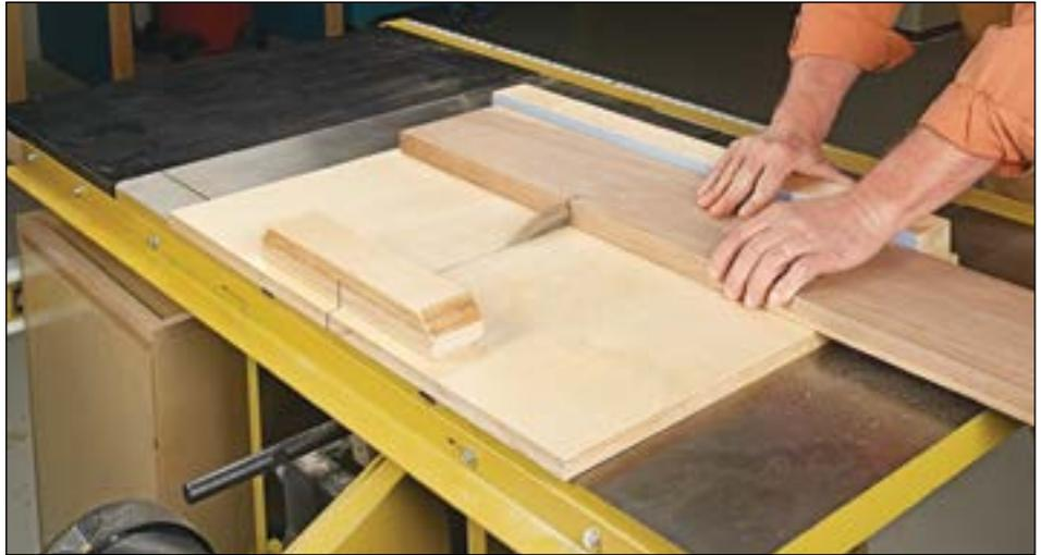
This crosscut sled allows you to cut boards or small panels to length. To build the sled, start by cutting the base to size out of a piece of  $\frac{3}{4}$ " plywood and radius the corners (drawing below). Then make a couple of hardwood runners to fit the miter gauge
