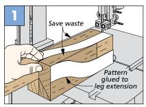
**First Cut.** With the patterns glued in place, make the cut on the underside (back) of the legs. Save the waste.
