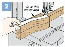
**Second Cut.** This cut shapes the outer edge of the leg. Save the waste to hold the pattern in the next step.
