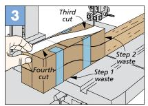
**Third & Fourth Cut.** Tape the waste pieces from the first two steps to the leg. Then make the final two cuts.
