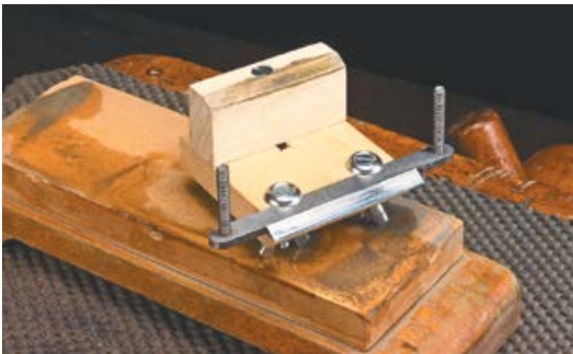
▲ A pair of finish washers hold the blade tightly in the jig allowing you to easily hone the cutting edge.
