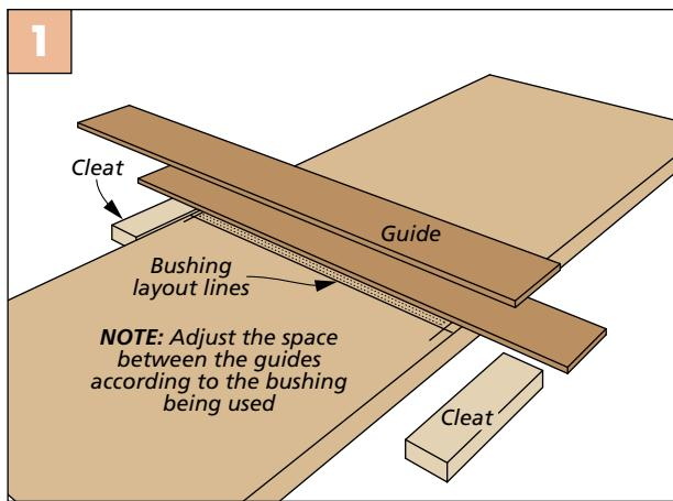
**Cleats Come First.** After drawing the location of the dado on the workpiece align the guides to the lines. Glue and pin nail the cleats to the underside of the guides.
