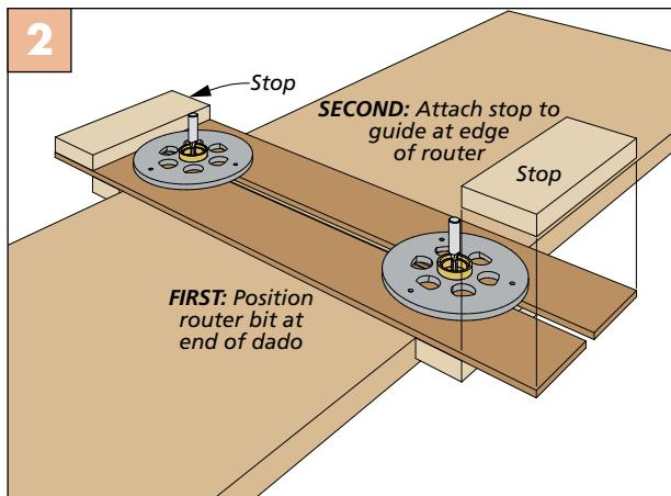
**Set the Stops.** With the router bit retracted, establish the stopping points at the ends of the dado. Use glue and pin nails (or double-sided tape) to hold the stops in place.
