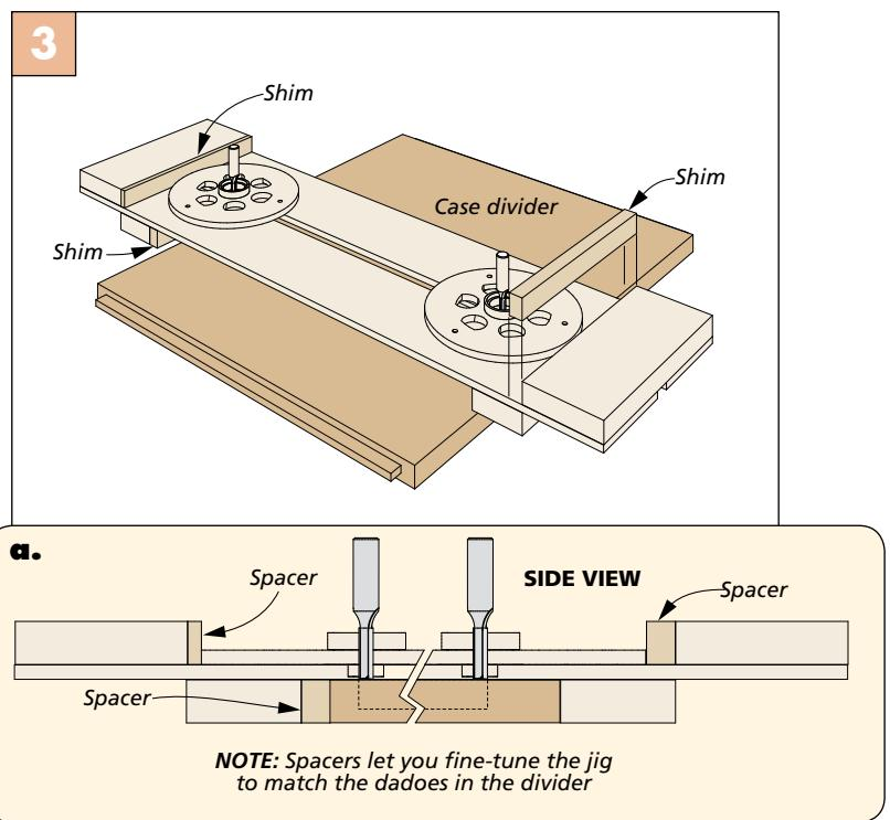
**Adjust the Jig.** The dadoes in the dividers are the same width and depth as the ones in the bottom, just shorter. Start by adding a spacer to the cleat, then add the two spacers to the stops to set the length and position of the dado.
