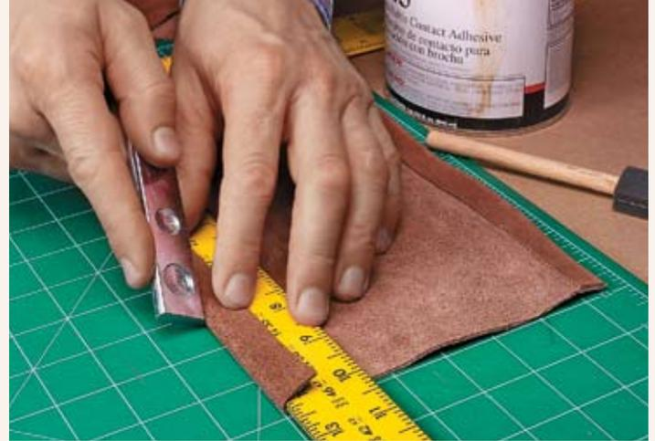
▲ **Folded Edge.** Rub the leather with a piece of metal to create a "crease." Then glue the mating faces with contact cement.
