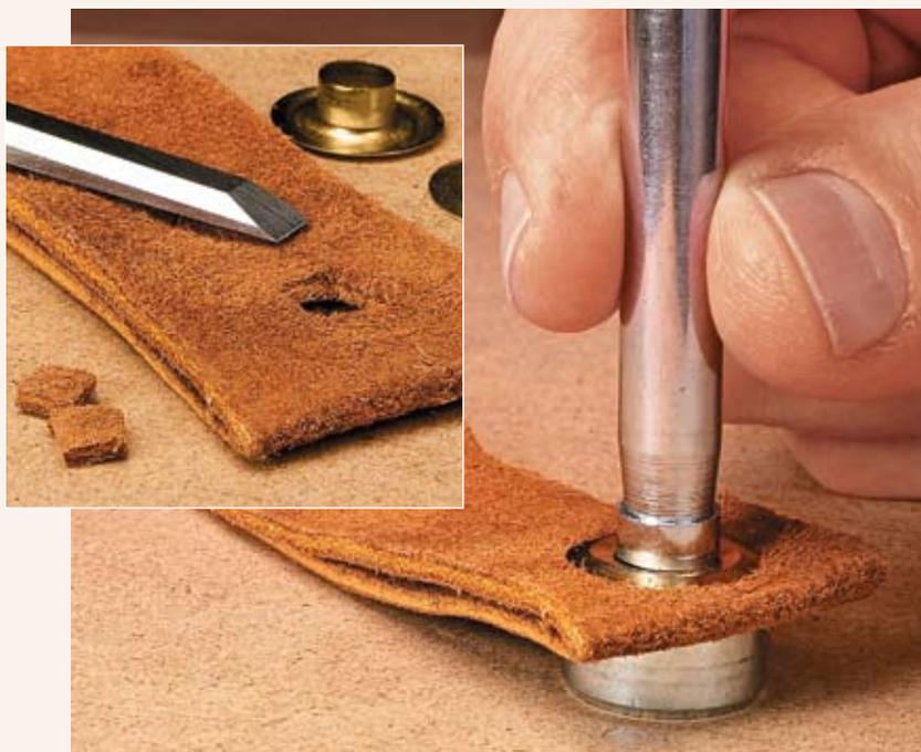
▲ **Setting Grommets.** You can quickly create an opening for a grommet with a few chisel cuts (inset photo). Then place the face of the grommet in the anvil and tap the setting tool to compress the stem.
