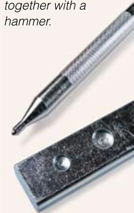
▲ **Rivet Tools.** The rivet setter is sized to match the rivet stem. The plate has dimples to accommodate several sizes of rivets.
