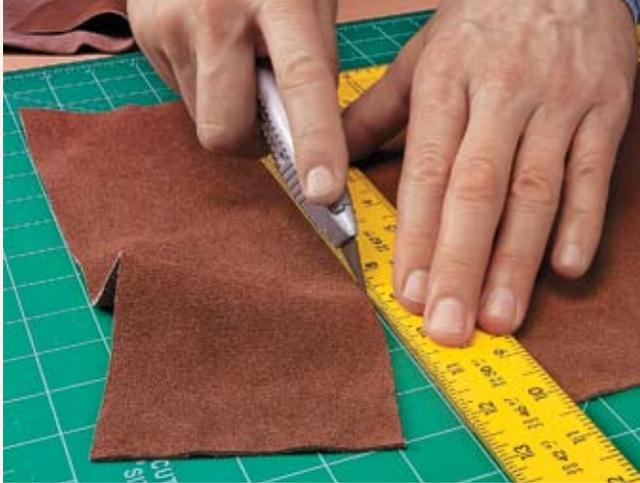
▲ **Cutting Leather.** A framing square guides a sharp utility knife as you cut through the leather in one pass.
