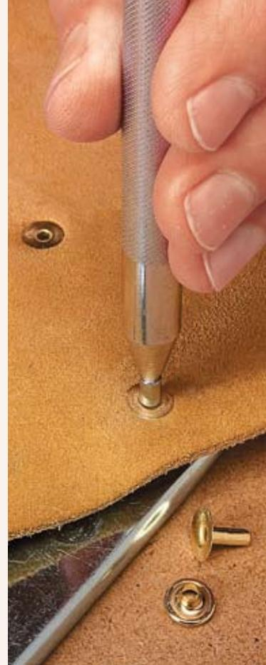
◀ **Riveting Leather.** Fit the stem through the hole and place it on the anvil plate. Place the washer over the stem and tap the pieces together with a hammer.
