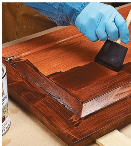
▲ Once the sealer is dry and the surface lightly sanded, brush or wipe on a liberal coat of glaze.
