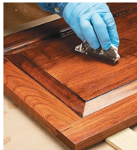
▲ Use a clean rag to wipe the glaze from the flat surfaces, while leaving remnants in the recesses.
