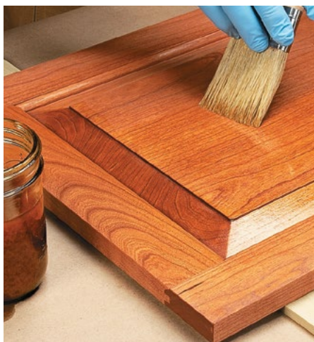
▲ After applying the initial stain, seal the surface thoroughly with a couple of coats of 1-lb. cut shellac.
