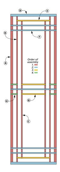
The grid work on the front of the tall clock is iconic for the Prairie style. It's a series of thin, narrow strips that are assembled with half laps and rabbets.
