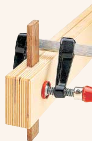
▲ A waxed “key” ensures proper alignment when gluing up the fence pieces.
