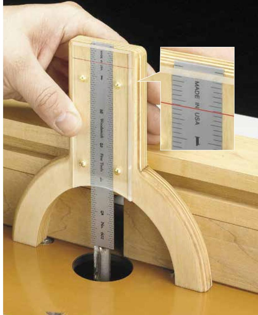
rests in a shallow groove cut in the gauge. This groove keeps the rule straight up and down during use.
