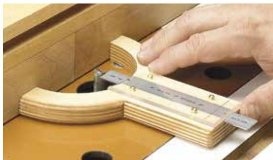
**Router Table Fence.** Setting the position of a router table fence can be a hassle. But with the set-up gauge lying on its side, it’s a simple, accurate task.
