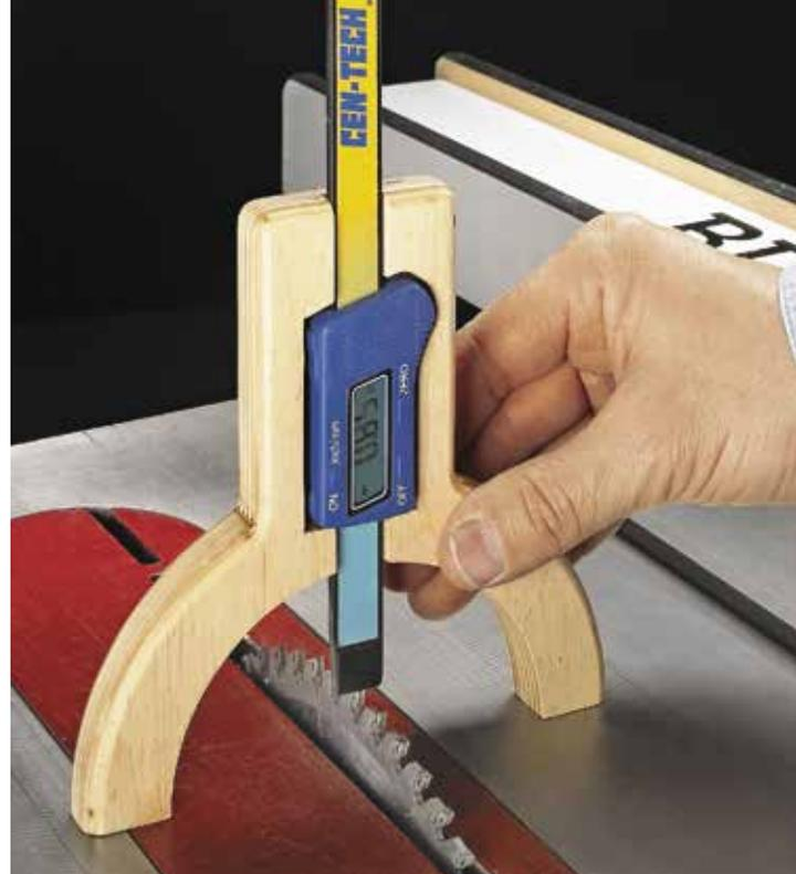
remains. Then use instant glue to secure the caliper into the cutout.
