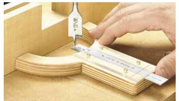
**Drill Press Fence.** In a similar manner, you can use the set-up gauge to position a drill press fence. This ensures that the drill bit is right where you want it.
