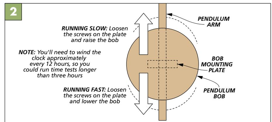
**Speed Up or Slow Down.** A simple way to check the speed of your clock's movements is to do a test run of three hours. At the end of the test, adjust the pendulum bob on the arm as shown in the drawing above.
