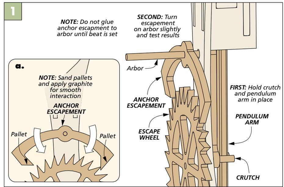
**Fuss & Fiddle.** The goal is to arrive at an even interval between the tick and tock of the clock. It's a trial and error process that involves slight adjustments along the way.
